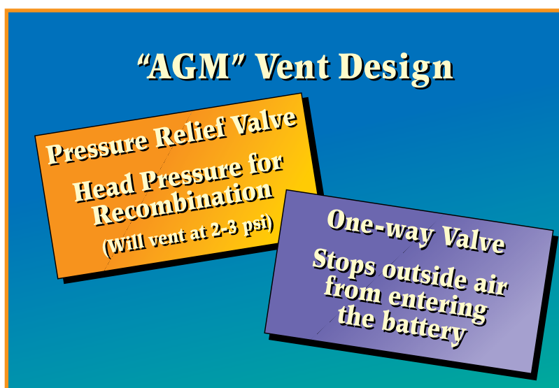
Figure C: One-Way Valve Allows Pressure Release. Characteristic of a Recombinant Battery System.
