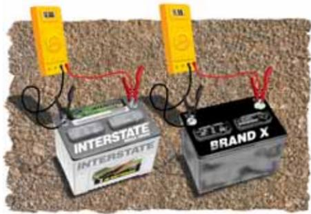
*batteries. To prove that the concrete myth was exactly that, we charged one on concrete and one on a 2x4 with the same charger for the same amount of time. The one on wood took a charge, and the one on concrete didn't! Very embarrassing.*
